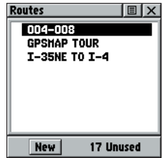
The Routes Page with a list of Routes and the number of Unused Routes.
